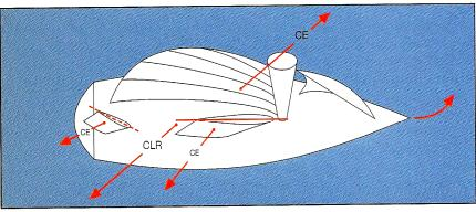
The center of effort (CE) is the position of the sum of all the lift and drag forces produced by the sails. The center of lateral resistance (CLR) is the equivalent position of all forces produced by the hull and its appendages. When the two centers are balanced against each other, the boat travels in a straight line (top). When they are out of balance, the boat turns. Changing the rudder angle (bottom) shifts the position of the CLR aft so that the boat turns to leeward.
